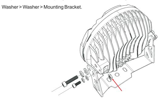
3. When mounting to the desired application, the order of the hardware is as follows: Bolt > Mounting Bracket> Rubber Pad> Mounting Platform> Washer> Spring Washer> Nut.
